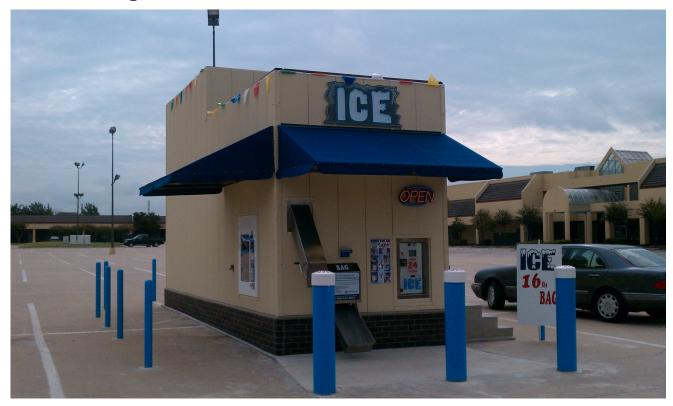
If you live in the southern part of the US, you've probably seen one of these ice vending machines. They are self contained manufacturing plants and retail stores, capable of producing 6,500 lbs of ice per day and dispensing packaged bags of ice automatically, all controlled by a single PLC.
